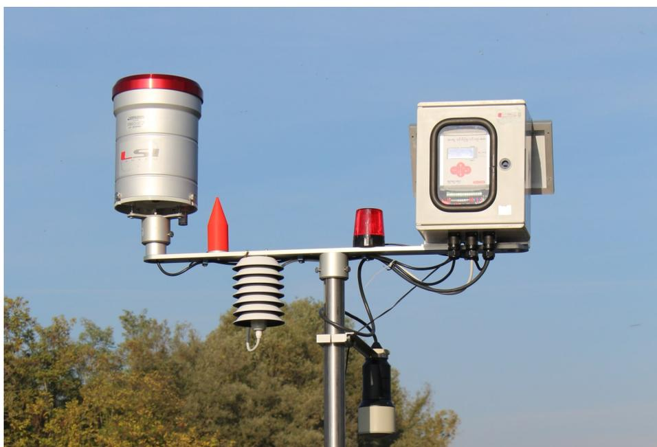
▶ The storm front distance sensor is particularly suitable to be connected to Alpha-Log (DLALA0100) or Pluvi-One (ELP001) data-loggers and mounted on the DYA046 bar (see figure), or fixed on the DYA032 mounting arm, to complete an early warning solution.
