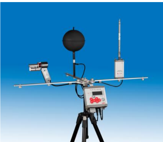
M-Log (ELO009) tripod mounting using a stand.
