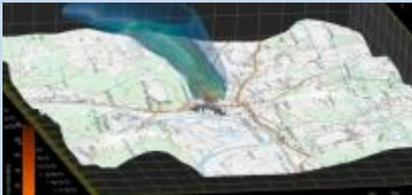
NUMTECH employs the very latest Gaussian dispersion models, such as ADMS or AERMOD/ISC, to produce studies for a wide range of industrial sites, while factoring in particularly complex effects such as hilly terrain, mixed land use patterns, obstacles, local weather conditions, etc. For sites with a particularly complex configuration, our engineers bring even more sensitive 3-D tools into play, selected according to the scales involved:
